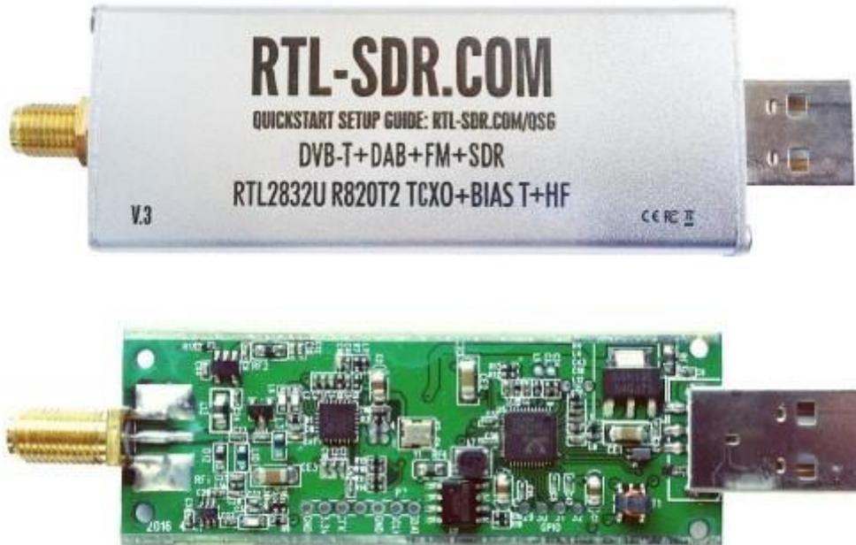
The RTL-SDR Blog V3 is an improved RTL-SDR dongle. RTL-SDR dongles were originally designed for DVB-T HDTV reception, but they were found by hardware hackers to be useful as a general purpose SDR. The standard dongles are okay for DVB-T reception, but are just barely suitable for SDR users/experimenters. The RTL-SDR Blog V3 was redesigned with SDR user needs in mind, instead of DVB-T HDTV users who typically have more relaxed requirements.
